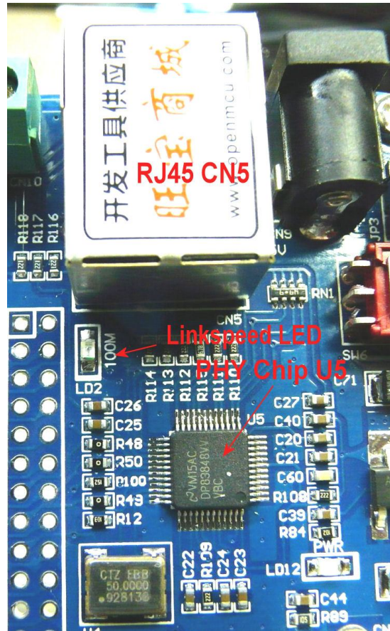
Figur 17 Ethernet PHY and RJ45 connector
