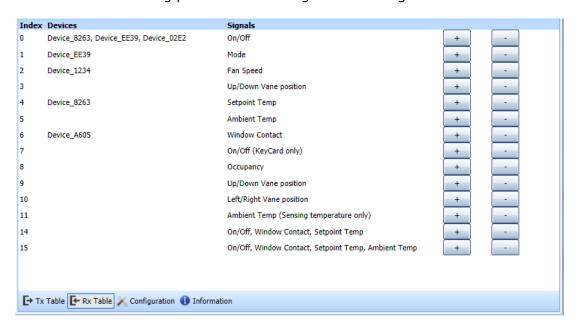
Figure 1.1 Reception channels with their associated signals and devices
