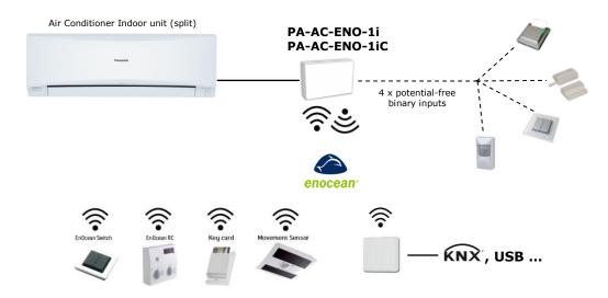
IntesisBox<sup>®</sup> PA-AC-ENO-1i allows monitoring and control, fully bi-directionally, all the functioning parameters of PANASONIC Air Conditioners from EnOcean installations.
