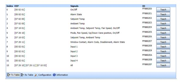
Figure 1.2 Transmission channels with their EEPs and unique ID's
