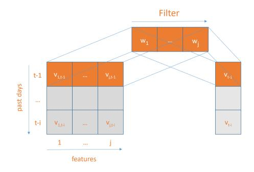
Figure 3: Applying a  $1 \times number$  of variables filter to 2D input tensor.
