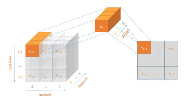
Figure 6: Applying a  $1 \times 1$  filter to the first part of the 3D input tensor.
