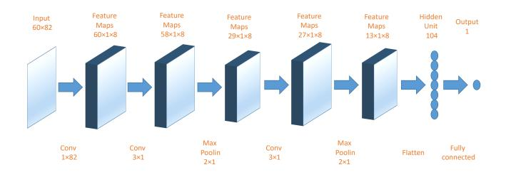
Figure 4: Graphical Visualization of 2D-CNNpred
