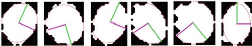
Fig. 5 Major and minor axes tracking
