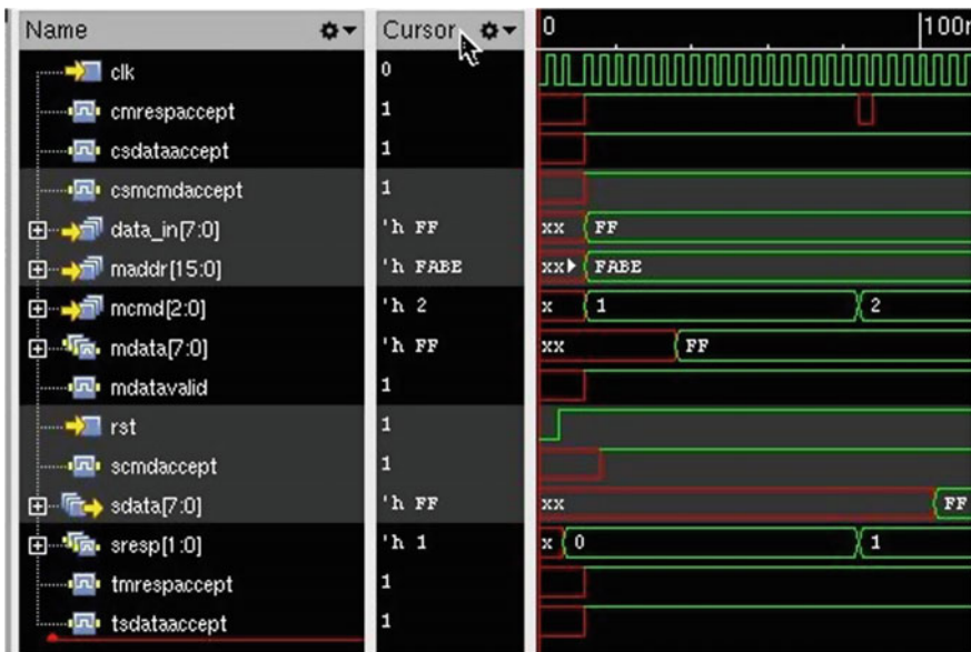
Fig. 6 Simulation results of basic mode OCP
