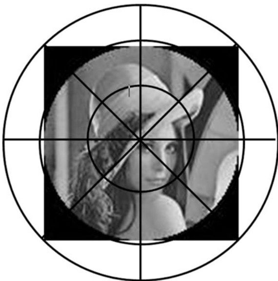
Fig. 1 Angular radial partitioning of an image to N angular and M radial sectors
