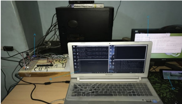
Fig. 4 System prototype (A: Sensor network with VLC Transmitter, B: Display of Transceiver python script running on BBB, C: Cloud Server running remotely, D: Web Application UI)
