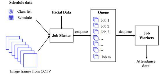
**Figure 5.** Archived image frames from CCTV are divided into jobs and stores in the queue for next process.
