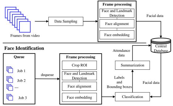
Figure 6. Components of an Ai processing unit.
