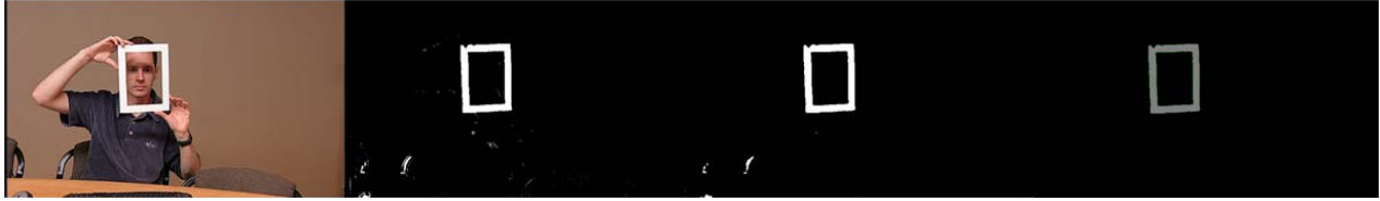
Figure 2: Target finding stages: Source, Color Match, Threshold/Filter, Region growing
