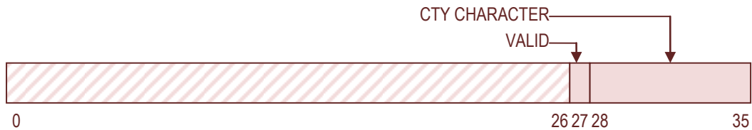
Figure 56 – KS10 CTY Output Word (KS10 Memory Address 000033)
