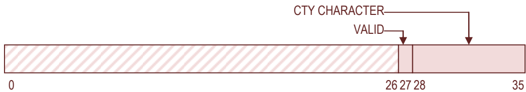
Figure 55 – KS10 CTY Input Word (KS10 Memory Address 000032)
