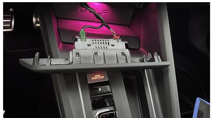
At the rear, the USB module can be replaced 1:1.
