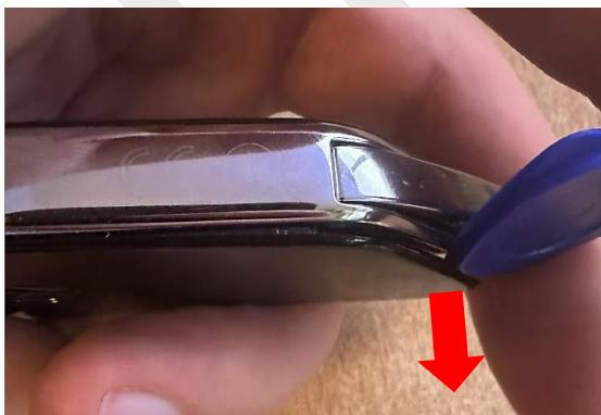
Insert the screwdriver between the two retaining tabs, push the battery slightly away from the tabs, and lever it out.
