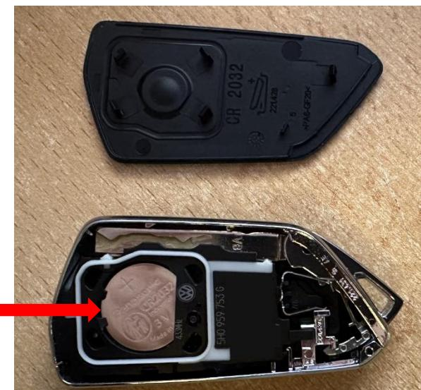
Insert the new battery and snap the cover back on.
