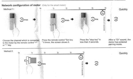
Press the motor's "Set key" 3 times in less than 5 seconds
