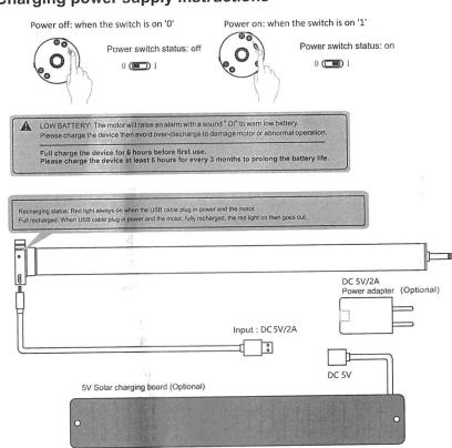
X When charging the motor, it is necessary to use the factory-configured charging cable to charge.
