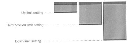
XThe up limit and the down limit must be set before the third limit is set, and the third limit will be deleted automatically when the up limit or down limit is deleted.
