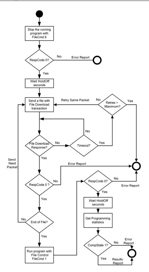
Use the File Control Command with a FileCmd parameter of 0x08 to stop the program currently running on the datalogger.
