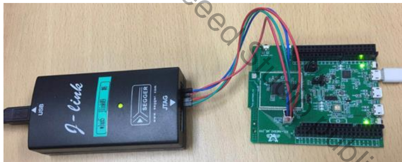
Fig 6-3 J-Link and Ameba-D SWD connection
