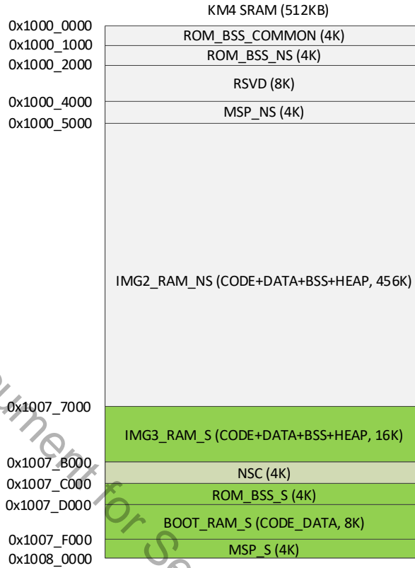
Fig 9-5 KM4 RAM program layout
