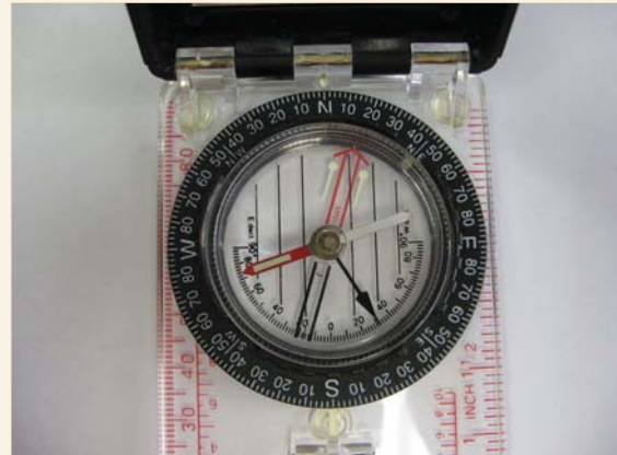
Figure 3-4a: A quadrant compass is divided into 4 quadrants, each reading from 0° (north or south) to 90° (east or west).
