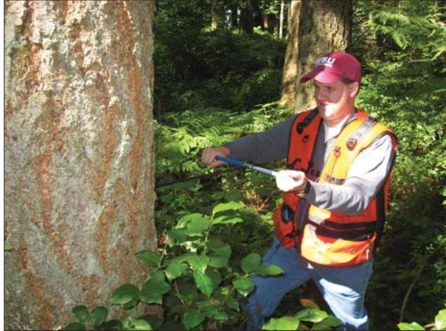
Figure 6-13: When using an increment borer, drill in straight toward the center of the tree at breast height.
