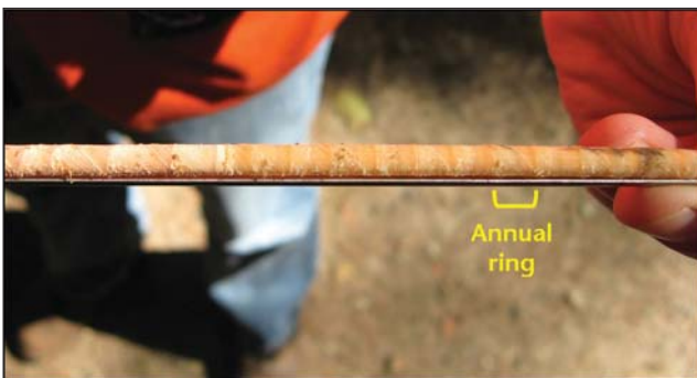
Figure 6-10: An increment borer allows you to extract a small core sample from the stem of a tree, from which you can determine the tree's age by counting the annual rings.
