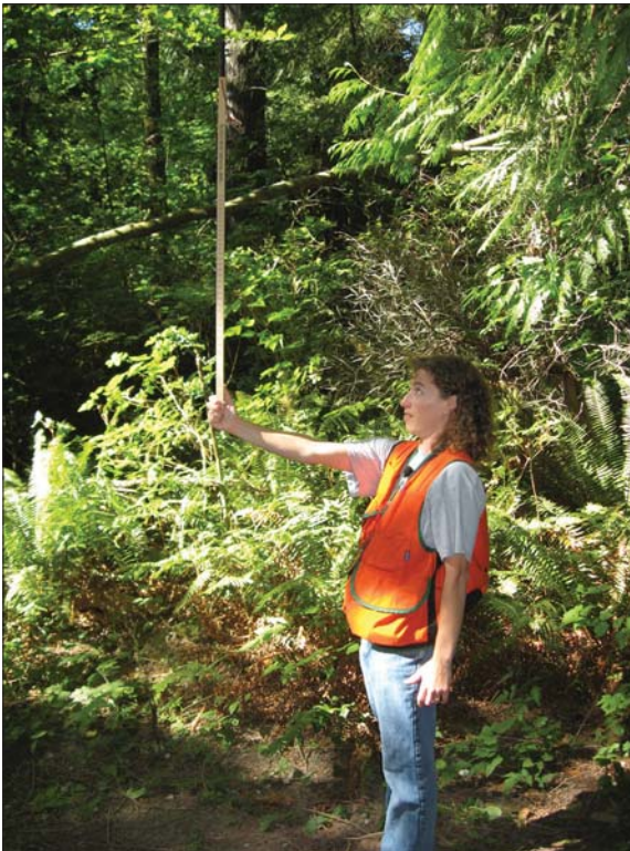
Figure 6-7: When measuring tree height with a woodland stick, hold the stick 25 inches from your eye and keep the stick vertical.
