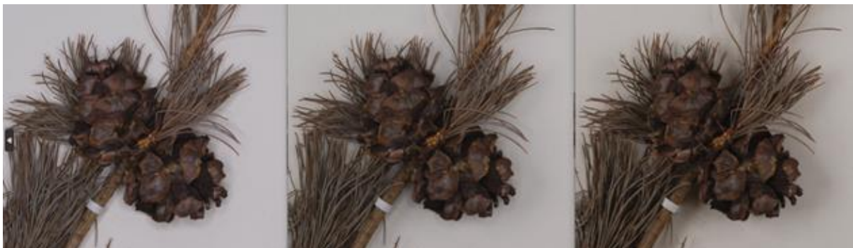
Fig. 4: Images of “thick specimen” lit using ringlight, ringlight+panels and panels respectively. Focus mode c. Aperture 4.5. GF 63mm f/2.8 R WR. “Aperture ring” off.
