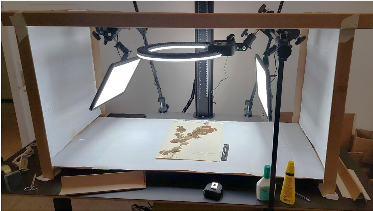
Fig. 3: Lightbox prototype with both ringlight and light panels.
