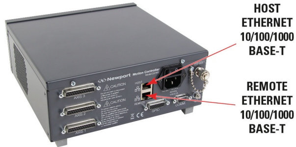
Figure 13: Direct connection to the ESP302 using Ethernet cable.
