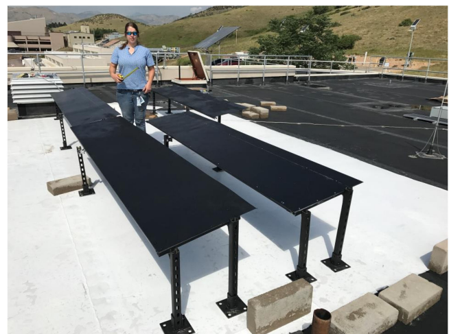
Fig. 3. Diagram (top) of the field test bed built in Golden, CO, USA, with two front-facing and four back-facing irradiance sensors. The array can be modified for row-to-row spacing, tilt angle, and clearance height. Photograph (bottom) shows array under construction, ballasts, and the white roof coating.
