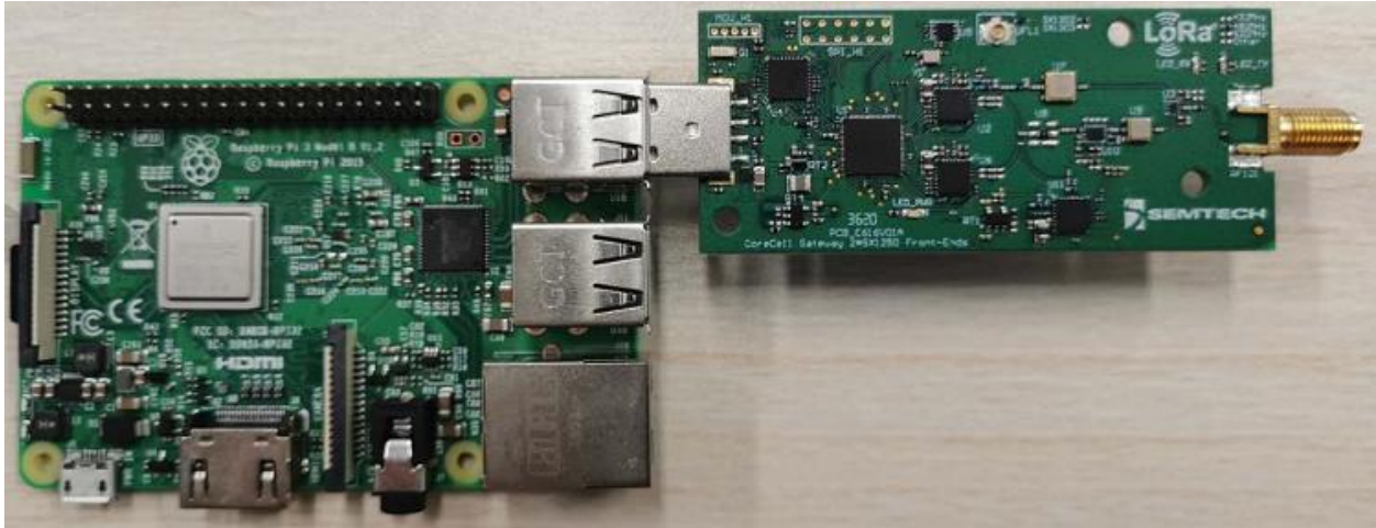
figure 4 The Corecell Ref. design mounted on the interface board with the RPI3
