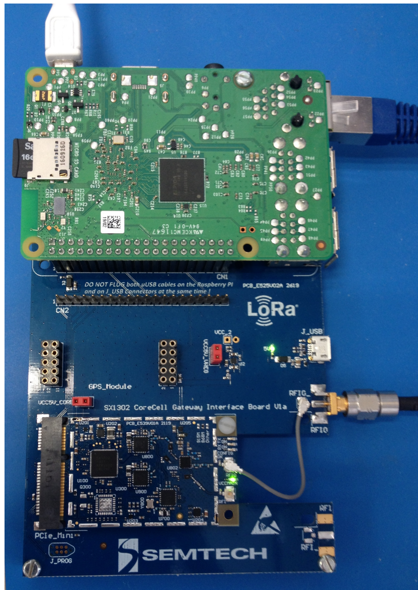
Figure 3.1: The Corecell Ref. design mounted on the interface board with the RPI3
