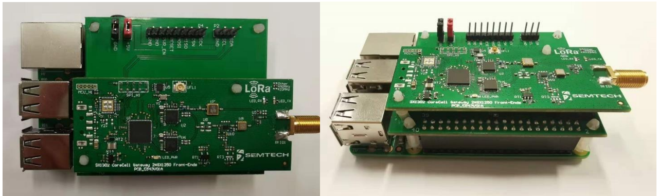
Figure 7: Corecell GW + interface board + raspberry pi Connection CN490
