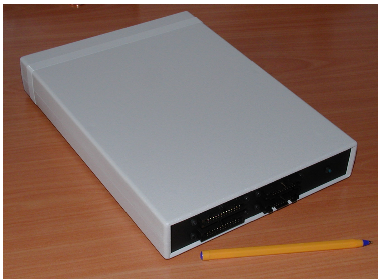
Figure 3: 40 channel high-voltage amplifier unit.
