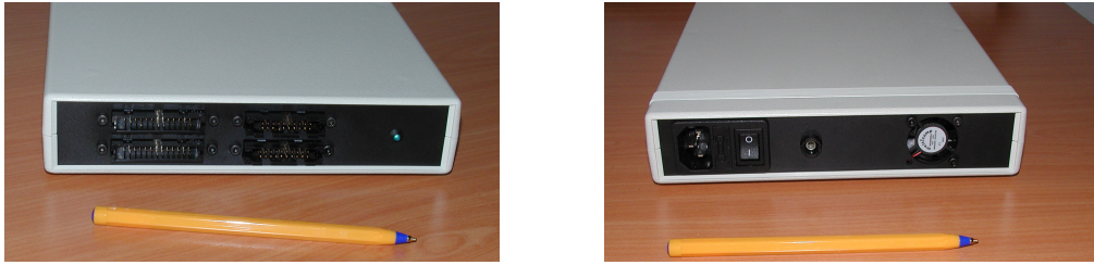
Figure 4: Front and back panels of 40 channel high-voltage amplifier unit.
