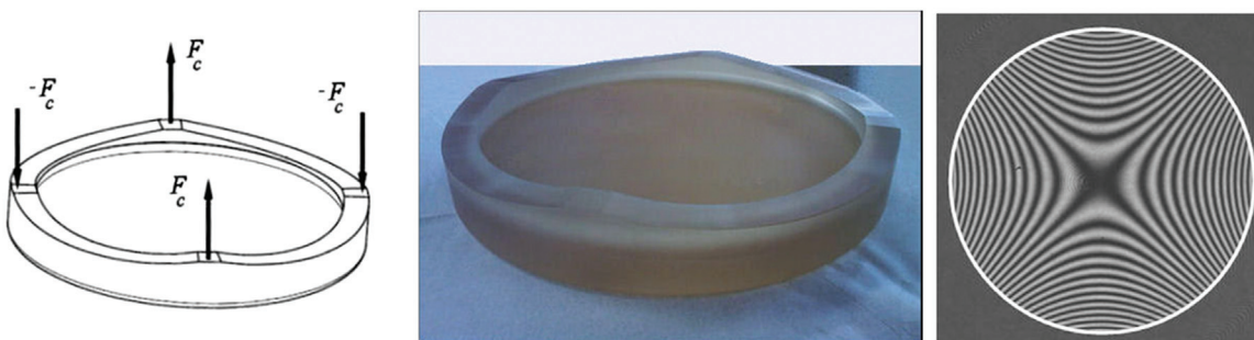
Figure 30 Left and center: Elasticity design in CTD class, i.e., t/t_0=\text{constant} , of a 40-cm mirror in Zerodur vitroceraam bent by four forces during stress figuring. Its contour realizes a built-in boundary to a ring whose axial thickness t_r(\theta) shows four azimuth thickness narrowings , t_{R-\text{Max}}/t_{R-\text{Min}}=1.16 , to ensure an accurate modulation in \cos 2\theta . Right: He-Ne interferogram with respect to a mean curvature sphere of one of the three Astm3 -correcting mirrors made for SPHERE. This instrument is a next-generation planet finder of the ESO-VLT (LOOM, Thales SESO Corp.).
