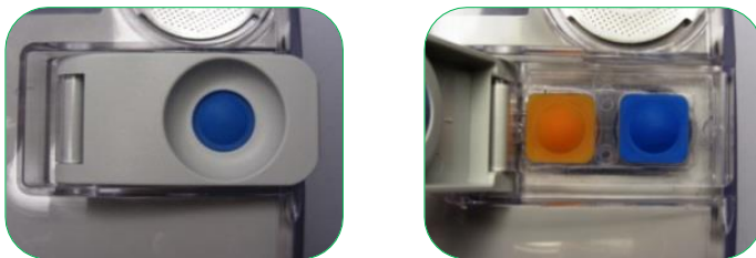
Figure 45: Scroll button (on the left) Reset and Scroll button (on the right)
