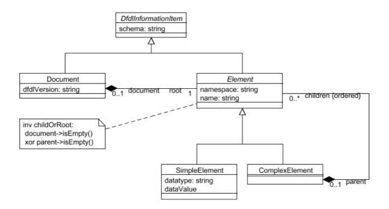
There are three kinds of concrete DFDL information item, Document, SimpleElement and ComplexElement. There are seven kinds of Nodes in the XDM, but when mapping from and to DFDL only four are used, Document Node, Element Node, Text Node and Namespace Node.
