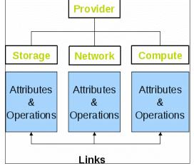
OCCI will be a very slim RESTful based API which can be easily extended. Without the overhead of many similar protocols the REST approach allows users to easily access their services. Every resource is uniquely addressed using a Uniform Resource Identifier (URI).
