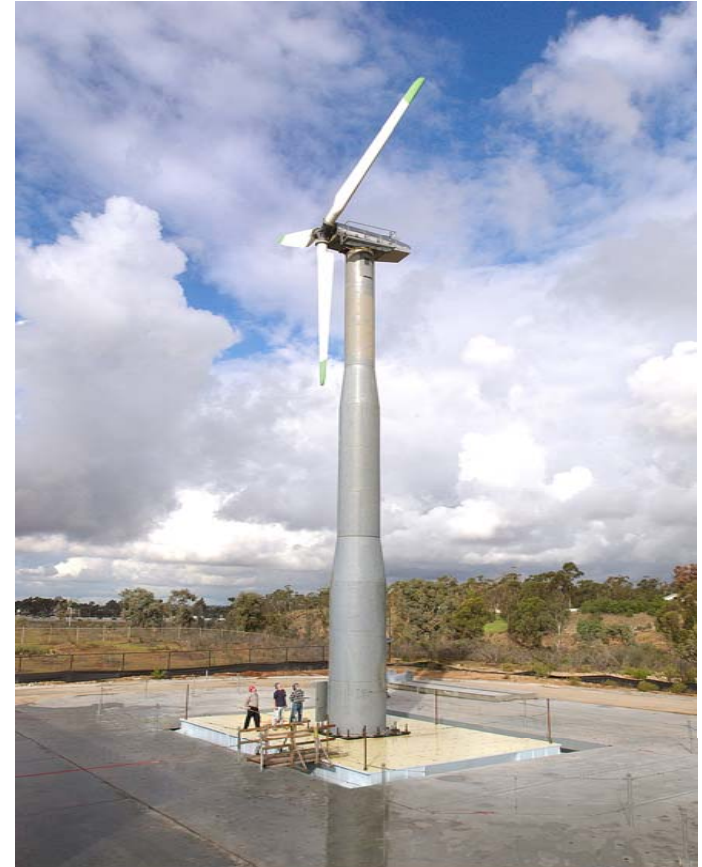
Pictured: Wind turbine test set-up on the UCSD-NEES Outdoor Shake Table at UCSD's Jacobs School of Engineering. The UCSD-NEES Outdoor Shake Table at UCSD's Jacobs School of Engineering is the world's first outdoor shake table and is capable of creating realistic simulations of the most devastating earthquakes ever recorded. The facility is part of the National Science Foundation's George E. Brown, Jr. Network for Earthquake Engineering Simulation (NEES).
