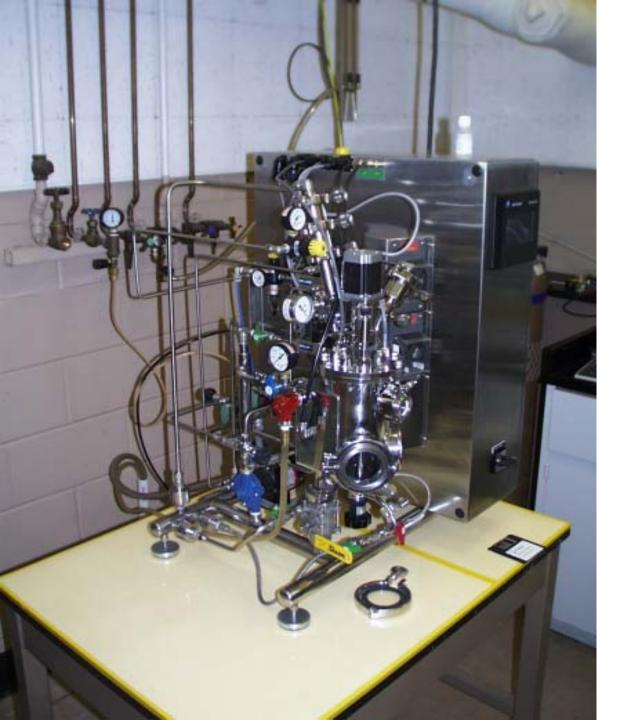
Here is the front view of the W.B. Moore's fermenter. It has two round glass windows for illumination of phototrophic cultures. One of them is seen at the bottom of the reactor steel vessel.
