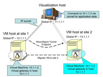
Figure 2. Tunnel migration for seamless external connectivity
