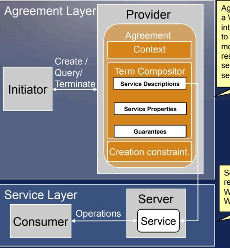
Agreement Layer: Provides a Web service-based interface that can be used to create, represent and monitor agreements with respect to provisioning of services implemented in the service
