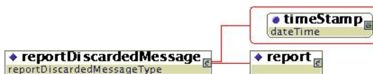
Figure 17: Schema for a message delivered when the repository discards incoming reports
