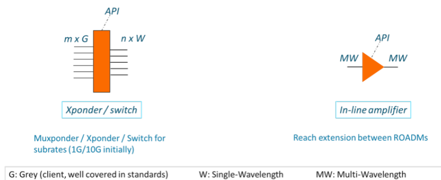
Figure 2: Switchponder and ILA
