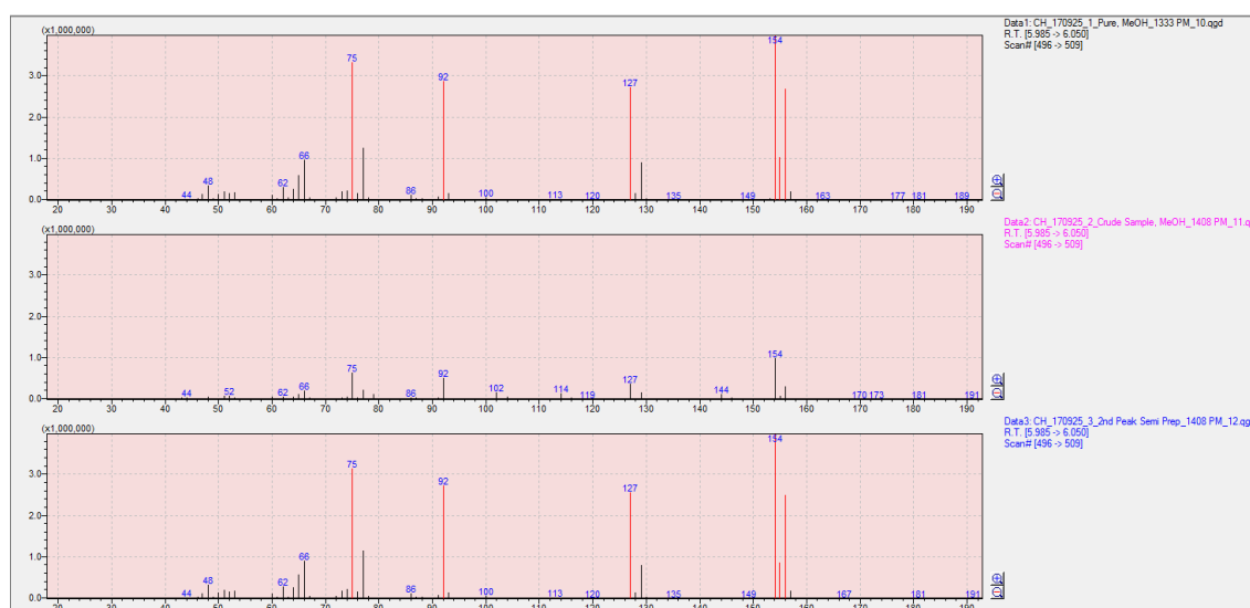
Figure X: Mass spectra of Crude reaction mixture, Pure sample and MTP Sample at R_t 6.02 mins peak
