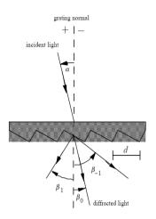
FIG. 1: Diffraction by a plane transmission grating. Adapted from [2].
