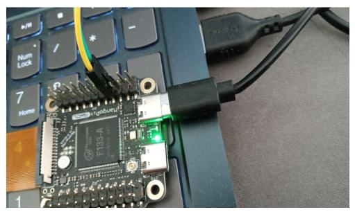
Finally, use the Putty.exe to connect to rt-smart's terminal using 500000 baud rate. Serial COM port numbers will vary depending on different machines. Device Manager to find out the exact COM port number respective to your machine.
