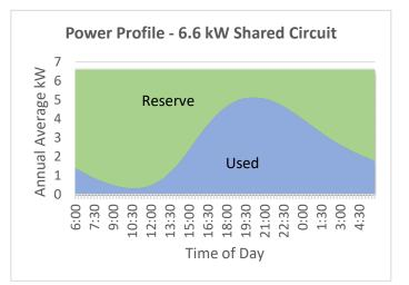
lower (per stall) than with dedicated circuits, because some vehicles will already be fully charged before that time. Overall efficiency is 41%.
