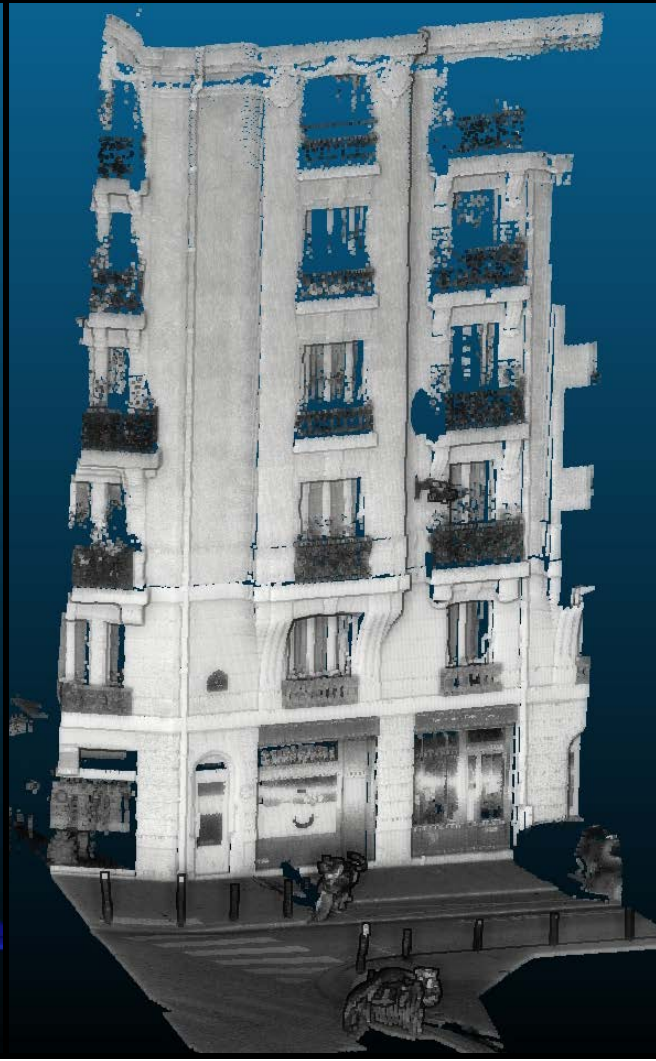
Point cloud colored with intensity of return
