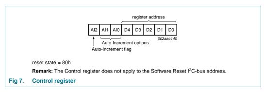
When the Auto-Increment flag is set (AI2 = 1), the five low order bits of the Control register are automatically incremented after a read or write. This allows the user to program the registers sequentially. Four different types of Auto-Increment are possible, depending on AI1 and AI0 values.
