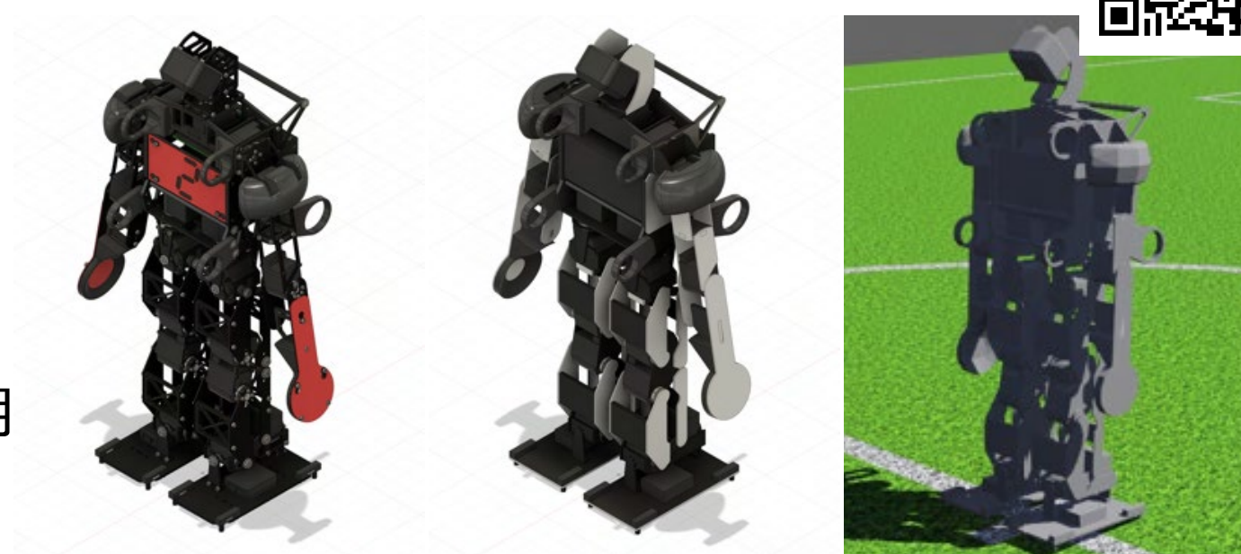
(a) 3D design model (b) Simplified 3D model (c) Webots model The 3D design model and simplified 3D model for the simulator of SUSTAINA-OP™
