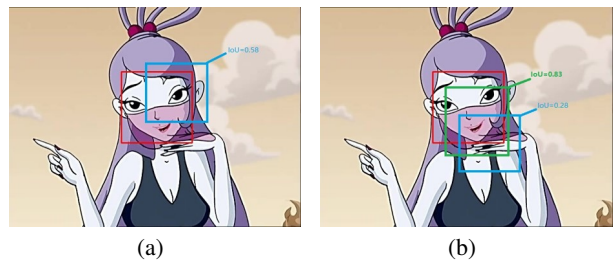
Figure 3: Illustration of our DAM, where red boxes mean ground-truth faces, blue boxes are anchors, and green boxes are the corresponding regressed bounding boxes. (a) Assigning anchors with IoU greater than the predefined threshold as positive samples, (b) assigning unmatched anchors in the first step with strong regression ability as positive.
