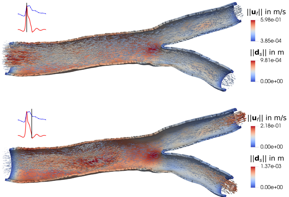
Fig. 16. Blood flow in an iliac bifurcation: fluid velocity vectors in the cut vessel geometry. Maximal inlet velocity at t = 5.31 s (top) and largest displacement and pressure at 5.49 s (bottom). The rapid decrease in the inflow velocity causes a flow redirection.
