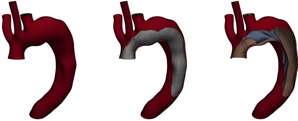
Fig. 1. Finite element discretisation of a dissected aortic arch: adventitia (red), media (peach) and flap (light blue) regions of the tissue and lumen (grey). Complete mesh (left), cut aortic arch revealing lumen mesh (middle) and cut aortic arch showing tissue elements only (right). (For interpretation of the references to colour in this figure legend, the reader is referred to the web version of this article.)
