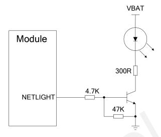
Figure 39: Reference Design for NETLIGHT
