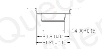
Figure 49: Tape and Reel Specification
