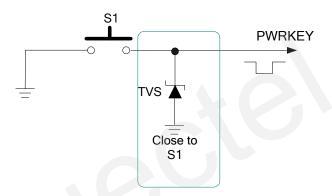
Figure 7: Turn On the Module with a Button
