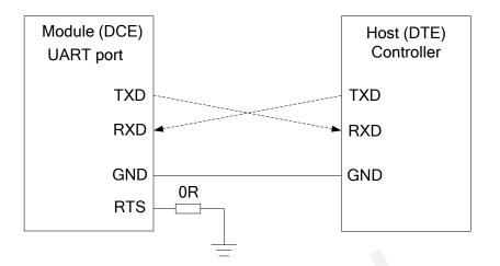
Figure 18: Reference Design for UART Port
