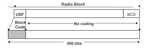
Figure 52: Radio Block Structure of CS-4
