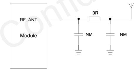
Figure 41: Reference Design for RF
