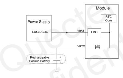
Figure 15: VRTC Is Supplied by a Rechargeable Battery
