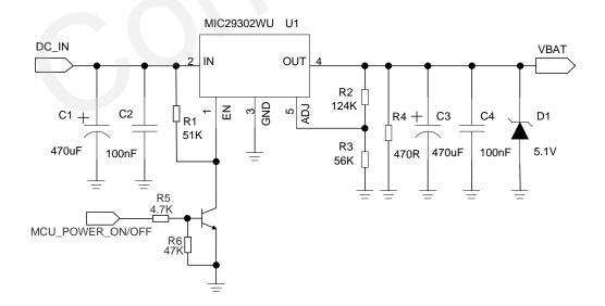
Figure 5: Reference Circuit for Power Supply
