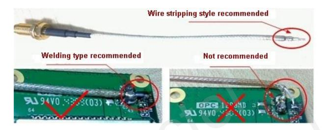
Figure 42: RF Soldering Sample
