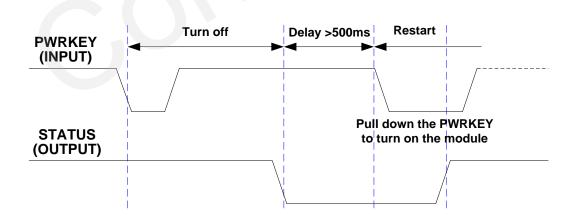
Figure 12: Timing of Restarting System
