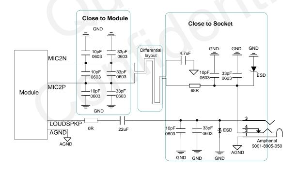
Figure 26: Earphone Interface Design
