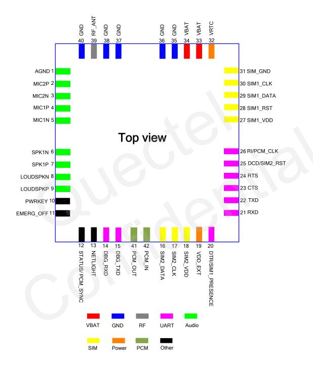
Figure 2: Pin Assignment
