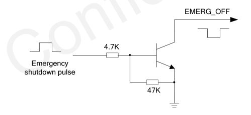
Figure 10: An Open-collector Driver for EMERG\_OFF
