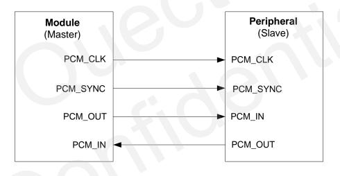
Figure 32: Reference Design for PCM
