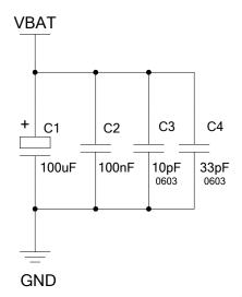
Figure 4: Reference Circuit for the VBAT Input
