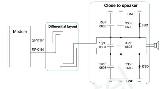
Figure 25: Reference Interface Design of AOUT1
