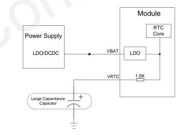
Figure 16: VRTC Is Supplied by a Capacitor
