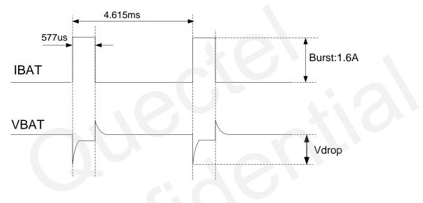
Figure 3: Voltage Ripple during Transmitting
