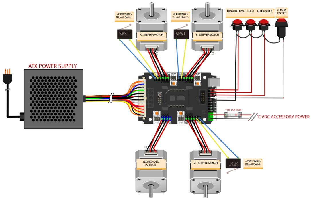
\* Fuse REQUIRED if connecting to 12VDC accessory output terminal (w/ ATX supply)
