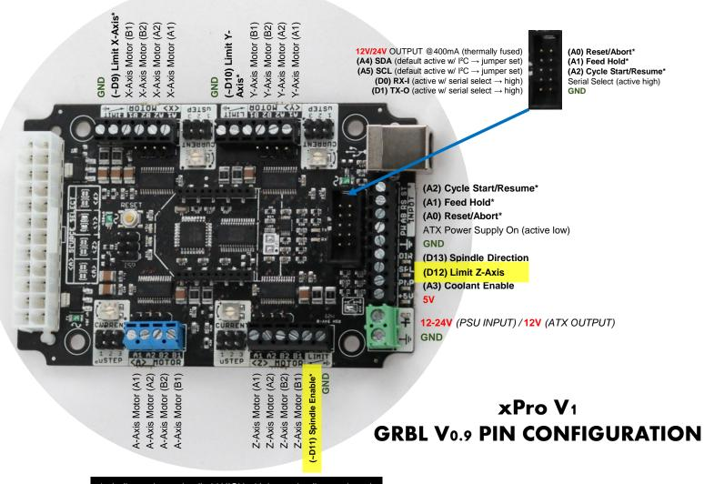
\* - Indicates input pins (held HIGH with internal pull-up resistors)
