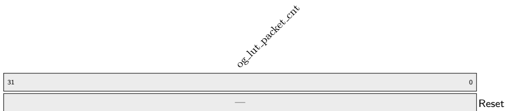
Register 22.39: UNOC_OG_LUT_PACKET_CNT_0 (0x00000230)
