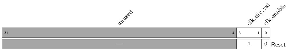
Register 21.12: ARM_CLK_CONF (0x000001bc)
