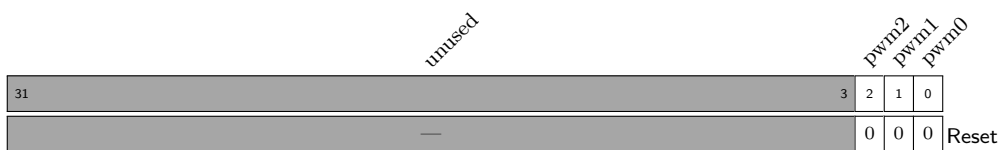
Register 21.57: PWM_ENABLE (0x00000050)
