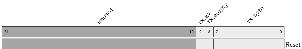
Register 21.45: SPLSU_RX_BUFFER (0x00000150)
