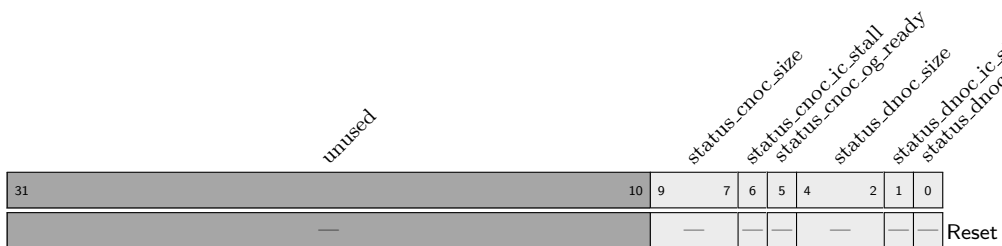
Register 22.17: UNOC_NOC_STATUS (0x0000006c)
