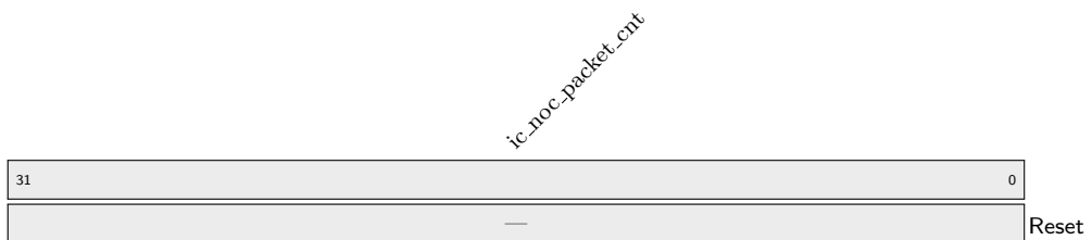
Register 22.41: UNOC_IC_NOC_PACKET_CNT_0 (0x000002f0)
