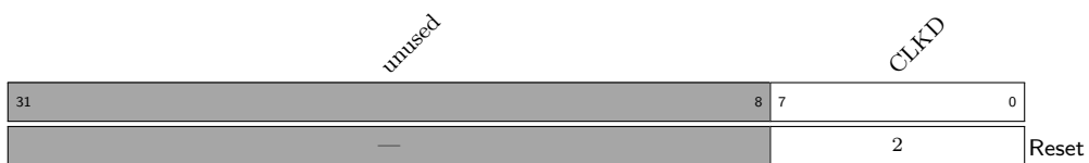
Register 21.76: SDC_CLOCK_DIVIDER (0x00000238)
