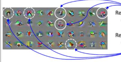
ResNet-34 learns three features (views) of a car: (1) front wheel (2) front window (3) side window
