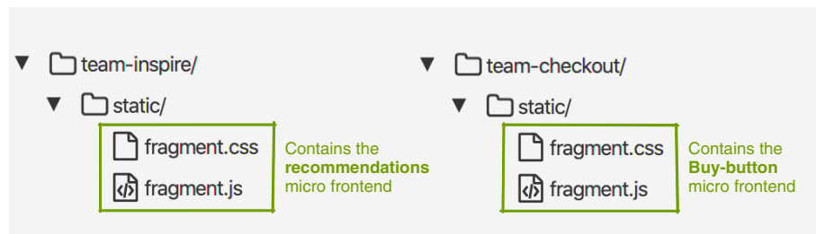
Figure 5.4 Both teams expose their micro frontends via CSS and JavaScript files that Team Decide can reference.
