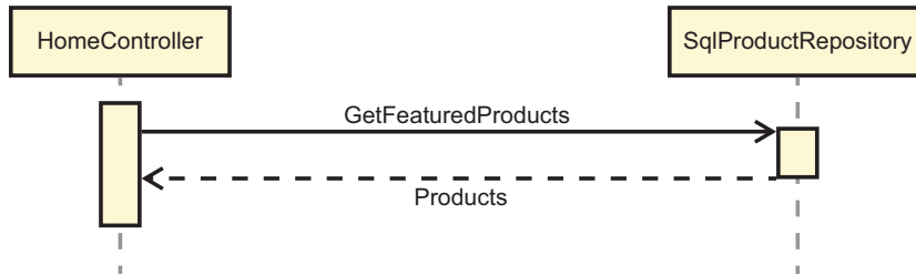
Figure 6.7 Compared to figure 6.6, removing the responsibility of managing IProductRepository 's lifetime together with removing the IProductRepositoryFactory DEPENDENCY considerably simplifies interaction with HomeController 's DEPENDENCIES .
