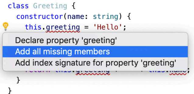
Figure 8-4. The quick fix to add declarations for missing members is particularly helpful in converting a class to TypeScript.
