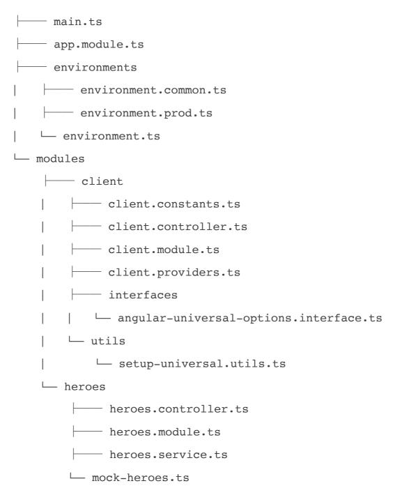
The modules directory will contain all of the Nest.js modules, exactly as we have seen in the previous section. One of the modules is the client module and will serve the Universal app and all of the required assets, as well as setting up the initializer to set the engine and provide some Angular configurations.
