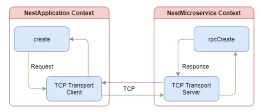
This diagram shows a simplified view of the data flow when a new user is created. The client makes a TCP connection with the microservice context and offloads the processing of the database operations. The rpccreate method will return a successful response with some data or an exception. While the
