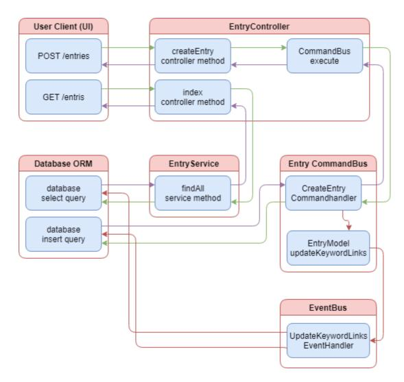
The above diagram provides a visual representation of how the entry command handlers work to keep the keywords updated. Notice how the flow of control is unidirectional. The command handler invokes the event using the entry model and then forgets about it. This is the asynchronous nature of the event bus in Nest.js CQRS.
