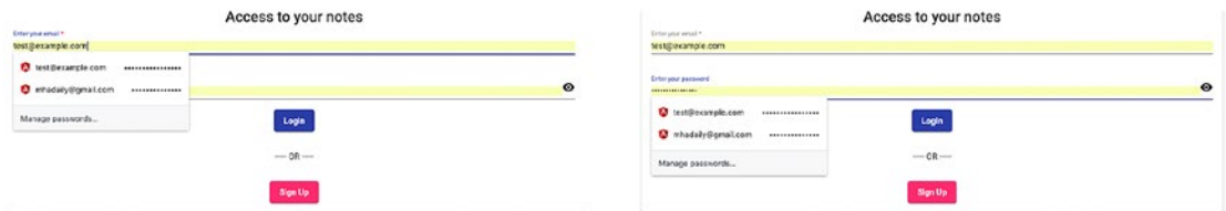
Figure 12-1. Autocomplete attribute allows browser to show appropriate username and password for the website
