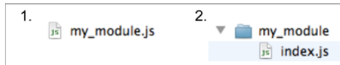
Figure 2.3 Node modules can be created by using either files (example 1) or directories (example 2).
