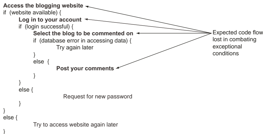
Figure 7.5 Expected code flow lost in combating exception conditions, without separate exception handlers
